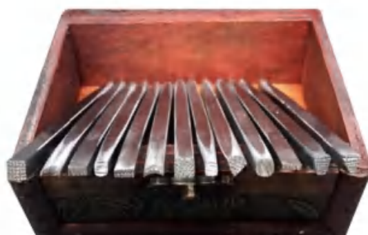
纹底整刀 Pattern bottom chisel knife TJK.00013 Φ5×90mm 13 Pcs
