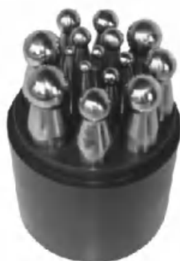
窝珠作 (冲头) 17支装 Dapping punches (17 Pcs) T.CG.00108 0.8kg 内腔尺寸 Cavity Size (mm): 2, 2.5, 3, 3.5, 4, 4.5, 5, 5.5, 6, 6.5, 7, 7.5, 8, 8.5, 9, 9.5, 10
